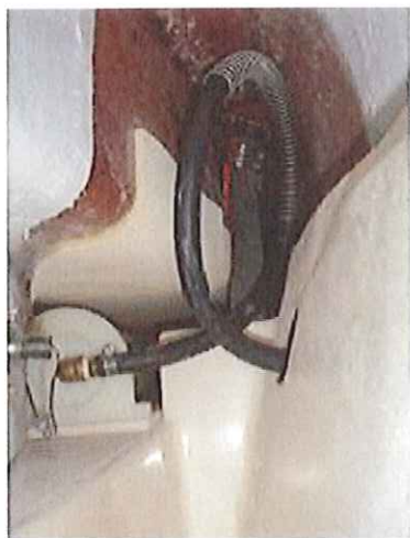
Inverted loop prevents water from entering canister
