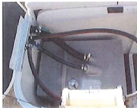
Fuel vapor separator prevents liquid fuel from entering the canister
